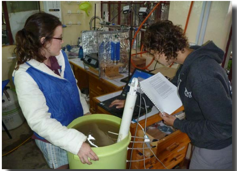
Kathleen and Hannah work on calibrating a soil moisture sensor in the Caylor Lab.
