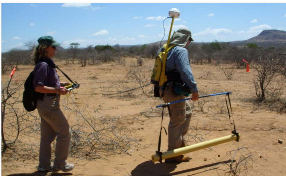
Trenton Franz and Lizzie King using electromagnetic induction to "see" where water is below the soil's surface. Photo by Joseph Kirathe.
