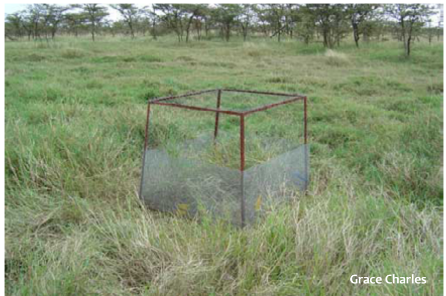
The productivity cages Grace and her colleagues used to measure how much plants grew over time.
