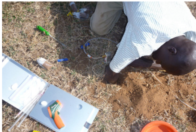
Ekomwa Akuwam sampling soil water vapor for isotope analysis. Photo by Keir Soderberg.
